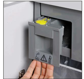
The EvenFlow Lubricator automatic oiler provides slow, continuous lubrication & ensures peak performance.
